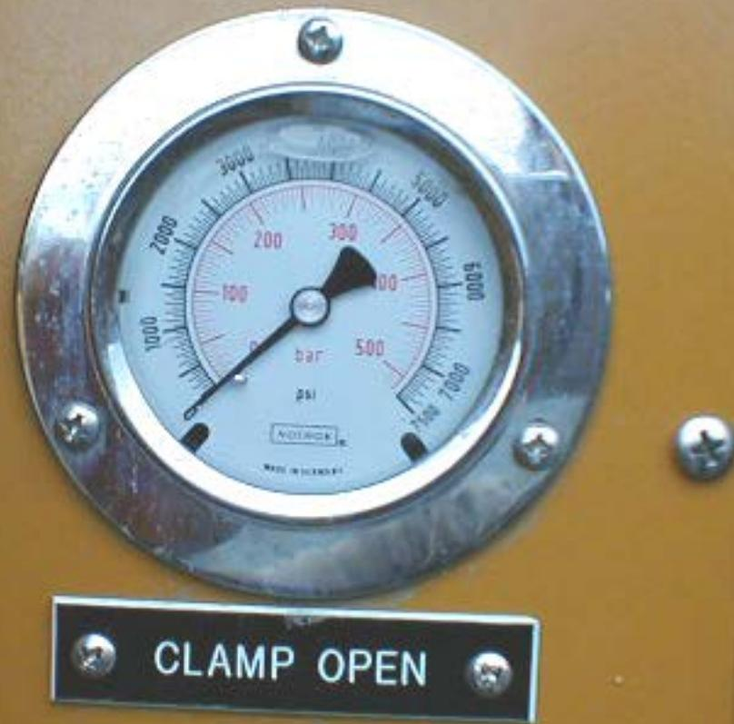
Clamp open reads the actual relief valve setting on the clamp manifold. You are reading the safety relief valve setting.
