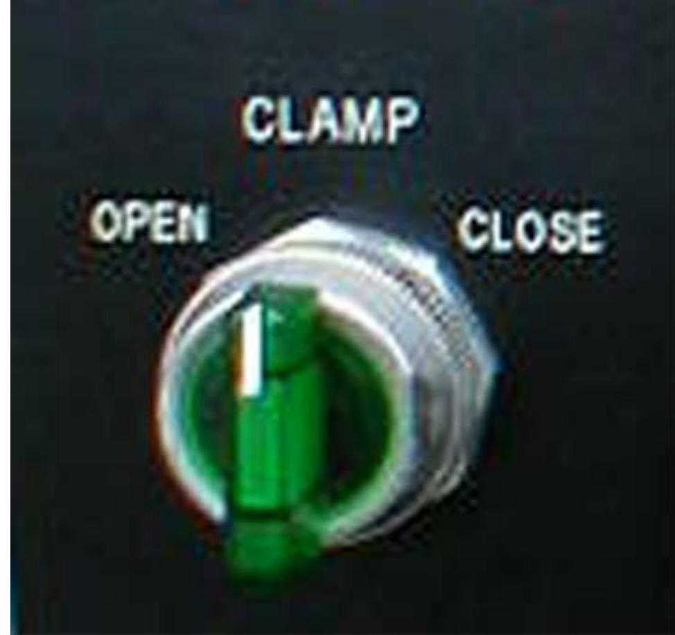
Switch is also a light. Light comes on when jaw pressure raises high enough to engage the pressure switch.
