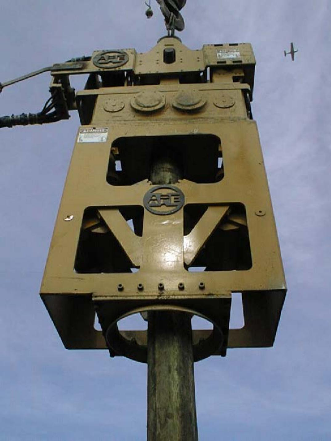
Center pull clamp has two jaws that are gear timed to make sure pile is centered. Designed for pipe up to 24", concrete piles, & wood piles.
