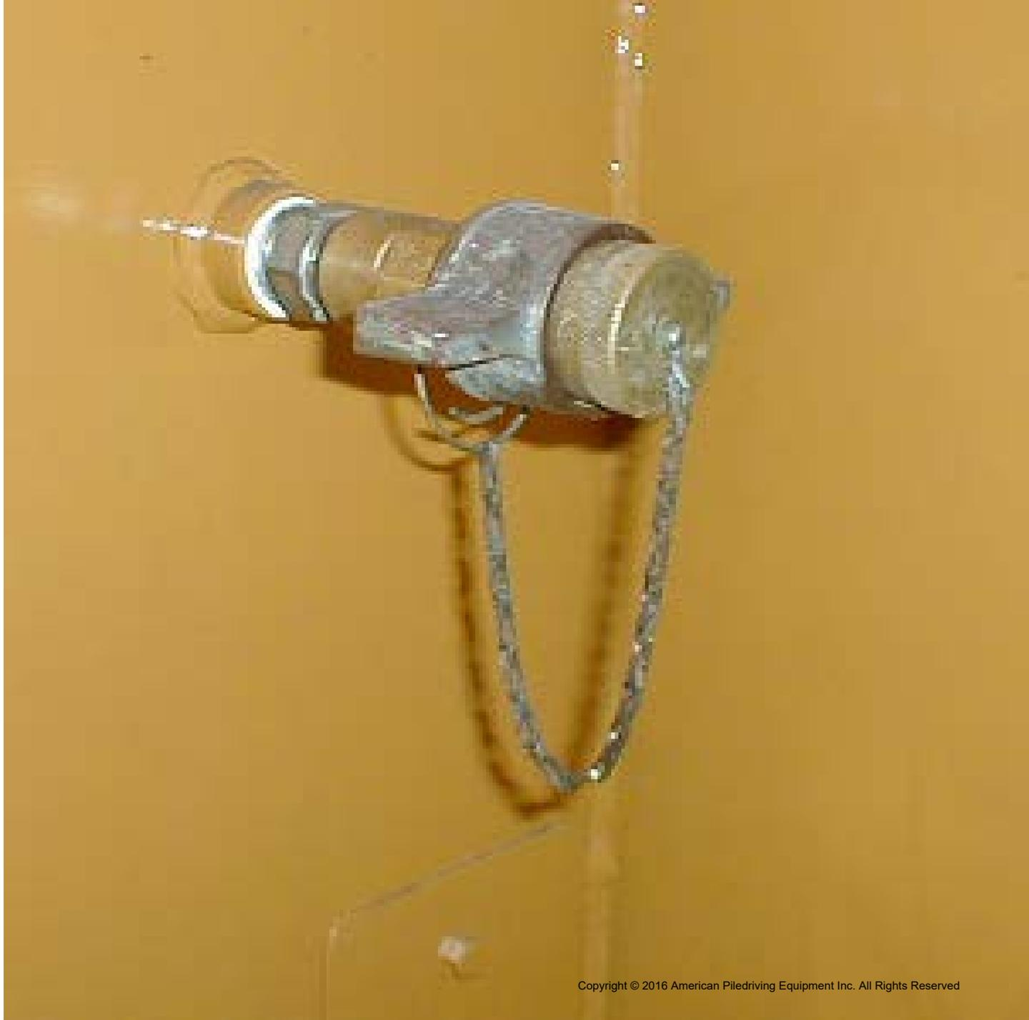
Control panel showing how power cables for solenoids can be removed quickly.
