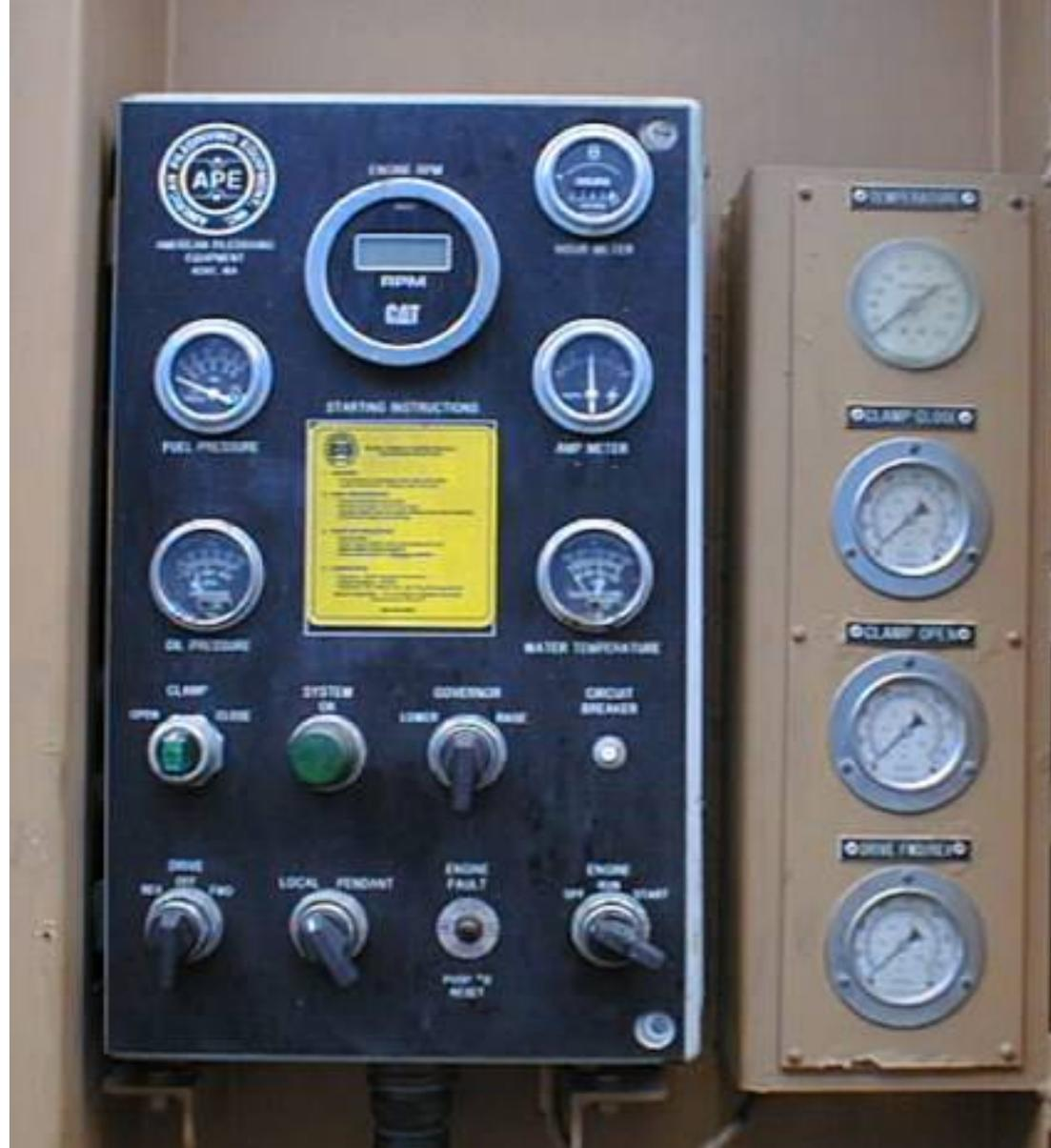
Same controls as on hand held pendant serve as back up controls if hand held pendant is damaged. Gauges show all pressures.
