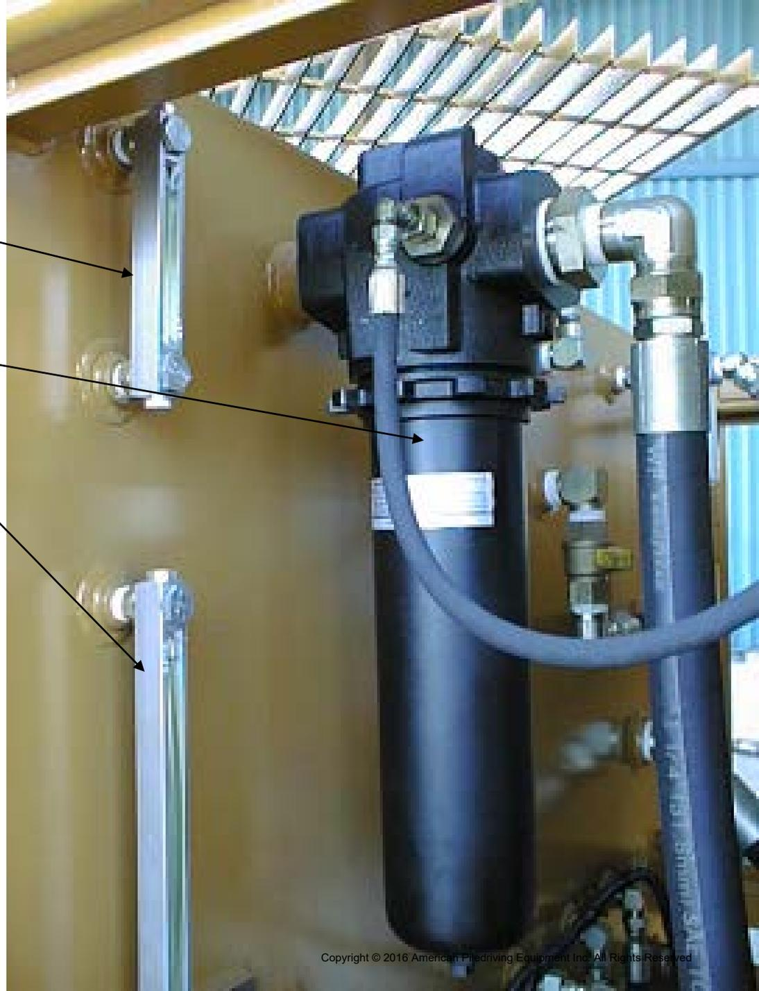
View of hydraulic tank level gauges and return filter.
